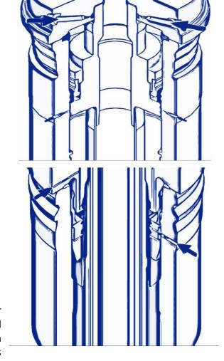
was performed. 30-minute pressure build-up tests were then successfully completed on each seal, confirming successful reinstatement of the 13-3/8" Pack- Off Seal, Tubing Hanger BT seal and Upper Hydraulic Packing/Lower Moulded O-ring. Q-Seal restored the integrity of every passing seal in the wellhead, providing full barrier isolation. The entire operation took just 5 hours.
